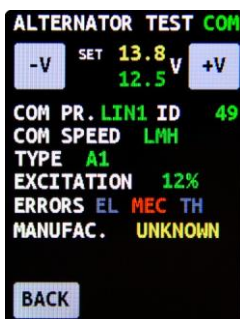
Fig. 7. Diagnostic window of the "COM"-type alternator.
